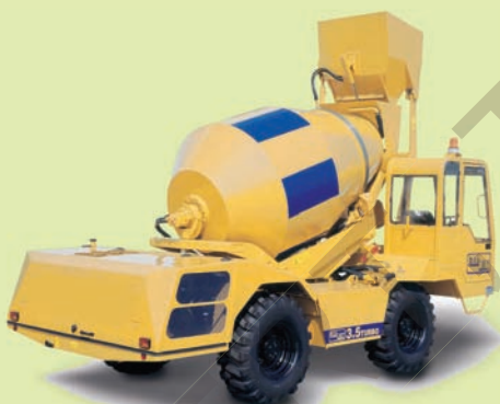
Mixer used for the concrete preparation
